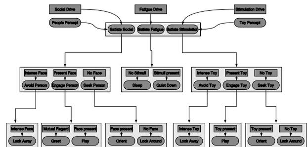
Figure 2: Kismet's behavior hierarchy. Only one behavior in a group is active at any given time.
